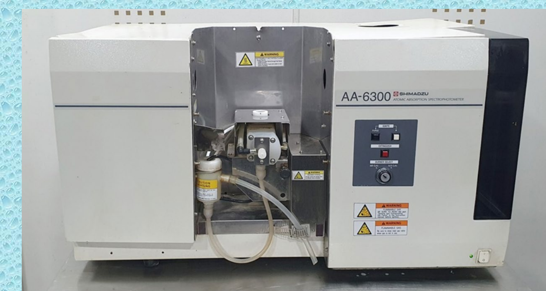
Figure 5 (above): Shimadzu atomic absorption spectrometer (AAS) with flame atomization for Cr concentration determinations.
