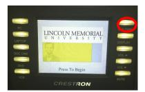
Press the PC button located below the power button to send the podium PC to the screen or if you are using a laptop, plug the cables in the podium to it and press the laptop button located on the left of the touch panel.
